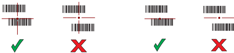
Figure 29 Pick List Mode with Multiple Barcodes in Aiming Pattern: Standard and Extended Range
